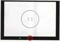
Compose picture and lightly press shutter release button. Confirm exposure indicator LED for background exposure.
