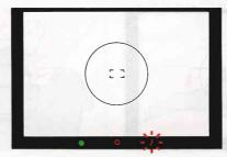
Recompose as desired, confirm ready-light is on, then fully depress shutter release button to take a shot with the flash.
